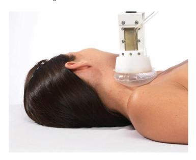
**MA-151:** mini-dual ridge wave guide applicators have an aperture of  $4 \times 5$  cm and individual heating patterns approximately  $2.5 \times 2.5$  cm by 2 cm deep. Advanced annular phased array principles create a central focusing of energy, which significantly overcomes the penetration losses of the energy radiated into the body.
