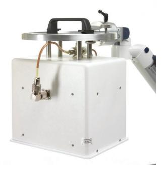
**MA-120:** side-loaded wave guide applicator has an  $18 \times 24$  cm aperture and a heating pattern of approximately  $12.5 \times 19.5$  cm by 2.5 cm deep.
