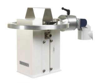
**MA-100:** side loaded wave guide applicators have a 10  $\times$  13 cm aperture and a heating pattern approximately 8  $\times$  10 cm by 2.5 cm deep.
